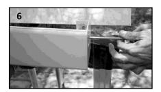
[STEPS 1-3] Start at one end of housing and remove 3 screws attached to housing and set aside. Repeat same process on other side of housing.
