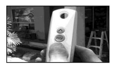
Using provided remote, lower shade down slightly by pressing down arrow. Put bottom rail back into pocket of fabric.
