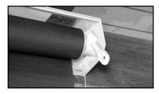
Before securing front housing, first rotate gear to lie vertical
