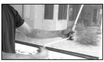
Slide hook end of hand brace into eyelet of gear on shade. Turn hand brace to rotate gear. Run shade up and down a few times to be sure there are no side rail adjustments needed.
