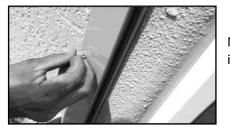
NOTE: Skip to step #6 if side rails are a side mount. Snap caps provided into mounting holes on side rails.
