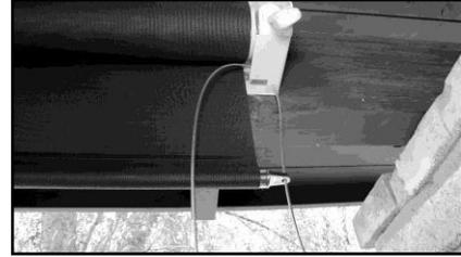
Slip cable up through the eyelet of bottom rail and push up through small hole in bottom of end cap. Continue pulling until top of cable is in reach for you to grasp. Using cable cutters, cut cable to proper length.
