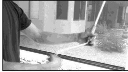
Slide hook end of hand brace into eyelet of gear on shade. Turn hand brace to rotate gear. Run shade up and down a few times to be sure there are no side rail adjustments needed.
