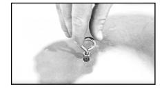
Thread eye bolt until it's tight and flush to the mounting surface.
