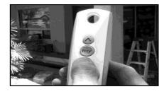
Using provided remote, lower shade down slightly by pressing down arrow.
