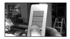
Using provided remote, lower shade down slightly by pressing down arrow.
