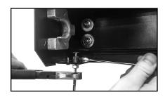
Hold cable sleeve while tightening the top nut using a 7/16 wrench.
