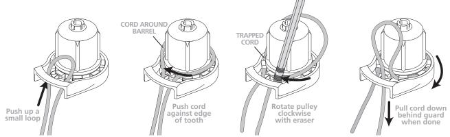
Push a loop up from behind the guard. Firmly push the cord clockwise against a tooth edge, until the pulley moves, trapping the cord in the pulley. Use a pencil eraser to rotate the pulley clockwise, one tooth at a time, all the way around to the other side.
