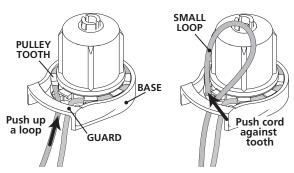
Hold the clutch by its base. With your other hand, push a small loop of cord up to the front from behind the guard.
