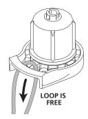
the pulley. Use the cord as a handle to pull the pulley all the way around until the cord is completely out of the pulley.
