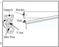
Set the post of the idler end into the V of the support bracket. Rotate the T-hook on the support bracket to lock in the post and secure the fabric roll.
