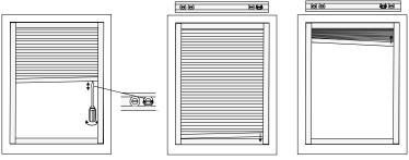
If the stack is uneven at the If the rail is uneven at the bottom, lower the high side top, raise the low side with with the outer adjustment screw.
