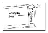
Allow the batteries to charge until the light on the charger turns green. A typical charge cycle can take between 4-6 hours.
