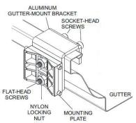
Securely attach rain sensor mounting plate to aluminum gutter mount bracket using flat head screws and nylon locking nuts. Slide gutter mount bracket over gutter lip and secure with socket-head screws.
