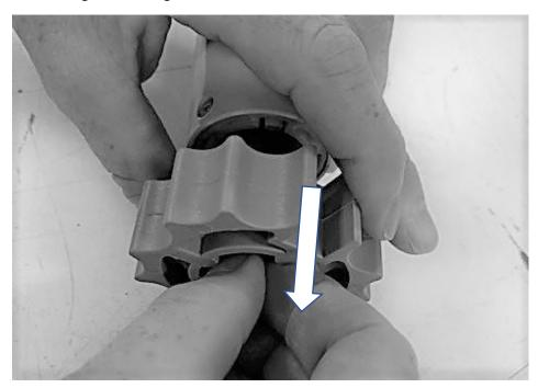
4. Slide new Drive on to the motor and ensure white tabs hold it securely in place.
