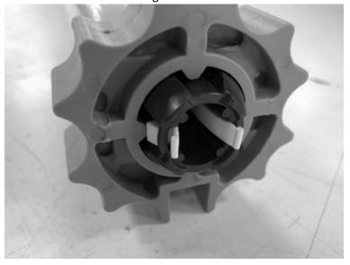
3. Holding the tabs together, slide the Drive off the end of the motor.
