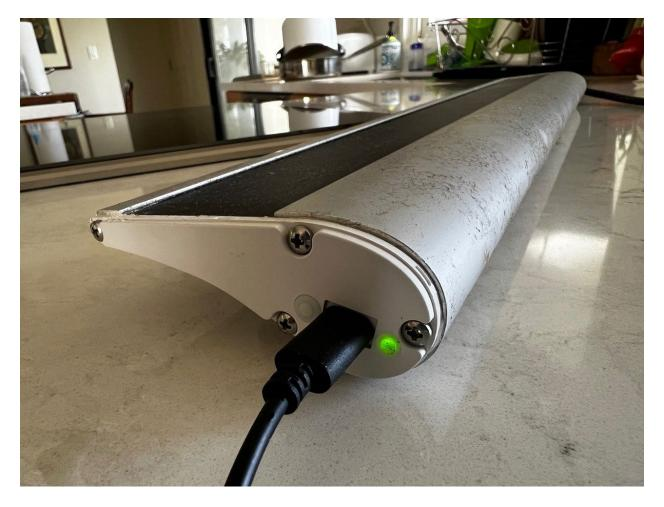
The USB port is underneath the end cap of the solar station on the end that does not have the cord coming out that attaches to the motor. You need to remove the cap to see it. The cap keeps water from getting into the port.
