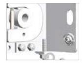
c. Finger tighten top nut. Leave approx.6 threads exposed above nut.
