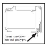
Step 2: Remove the end cap on the motor side, loosen motor screw and disconnect motor wire.
