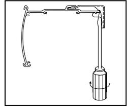
Twist the screwdriver until the head rail disengages from the bracket.
