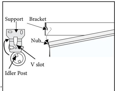
Set the post of the idler end into the V of the support bracket. Rotate the T-hook on the support bracket to lock in the post and secure the fabric roll.
