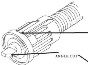
Drawing is spring mechanism not installed inside the roller.
