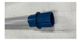
Slide all the way on to match notch on blue crown to motor. It must slip all the way on.
