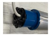
Slide in until both motor crown and drive are fully inserted into the roller tube. Then install the 4 screws to secure the motor crown on to roller tube.
