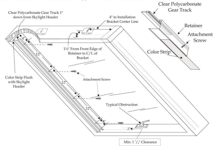
♦ Screw Installation Brackets into the skylite header with the center of the attachment screw hole 1¼" back from the front edge of the Retainer. They should be screwed four inches in from the left and right sides.
