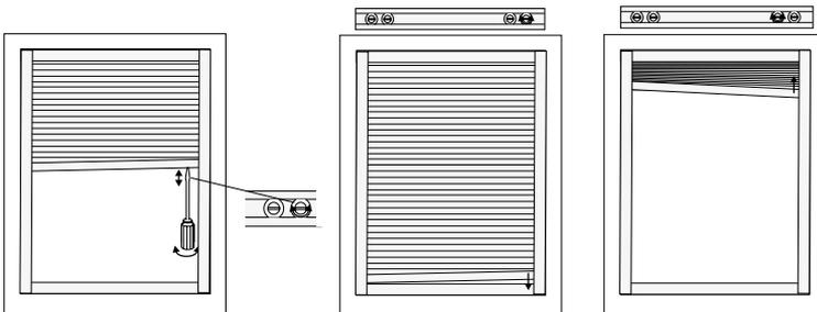
If the stack is uneven at the bottom, lower the high side with the outer adjustment screw.
