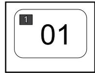
4. Confirm that the channel selected is set for bottom up only shades by looking to see if a number 1, 2 or 3 shows in the left of the display. If a number is shown, deactivate the Top Down/Bottom Up function for that channel by pressing the **RAIL SELECTOR** and **DOWN** buttons at the same time until the rail selector number disappears from the left side of the screen.
