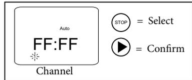
Use the **STOP** button to select the day and move on to the next one. Use the **UP** arrow to skip a day and the **DOWN** arrow to back up. You must press **STOP** for each day that you want to select. If the day is still flashing, it has not been selected.
