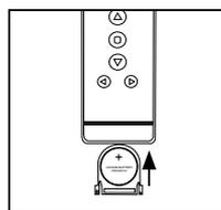
Insert the new battery (CR2430 lithium) into the battery tray so that the writing is facing up (positive up) when the remote is face up. Slide the tray back into the remote.
