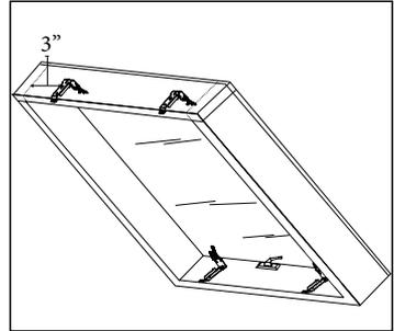
Using the installation bracket as a template, measure to the edge of the bracket and mark the hole locations with a pencil for drilling. When mounting brackets, make sure they are in line.
