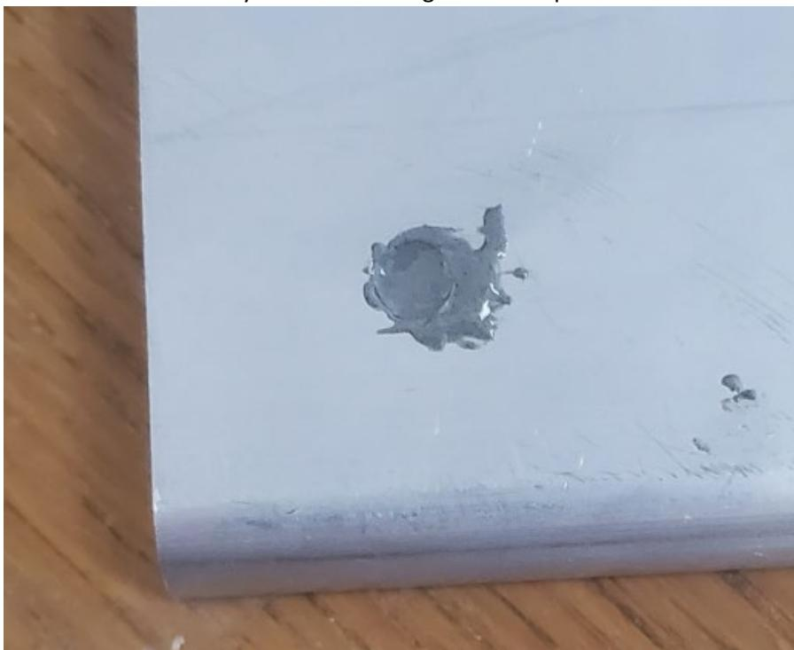
After the JB Weld cures (typically 24 hours), remove the electrical tape and see your patch:
